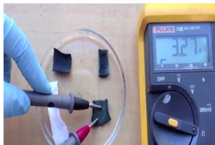
**Step 7d:** Test the doped (dry) PANI-treated fabric. Record result.
