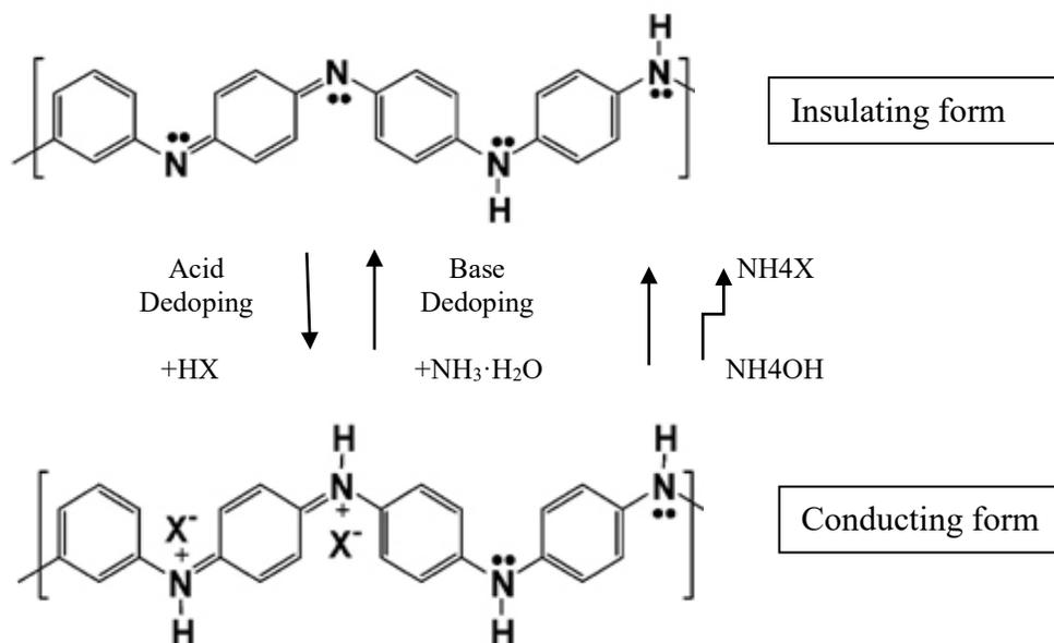
Figure 1. Reversible doping mechanism in polyaniline. HX= protonic acid
