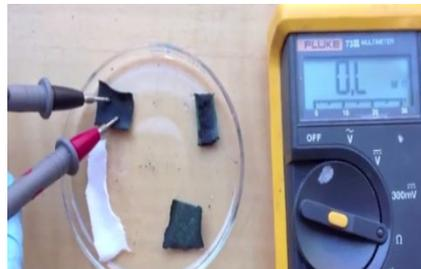
**Step 7b:** Test the de-doped PANI-treated fabric sample. Record its resistance.
