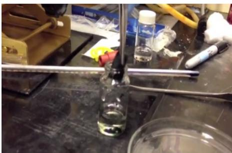
**Step 6:** Dip two of the dried pieces of cloth into hydrochloric acid to re-dope the polyaniline polymer. Gently dry one of the re-doped pieces of the fabric, which will cause the fabric to turn a greenish color indicating the polyaniline polymer has been re-doped. Keep another piece wet. Once doped fabric piece is dry, place the four pieces of fabric on a petri dish. One of each: untreated, treated de-doped, treated doped (wet), treated doped (dry).
