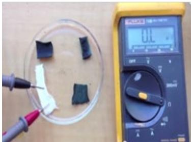
**Step 7a:** Measure the conductivity of the 4 cotton fabric samples. Begin with the untreated cotton fiber fabric square sample as the control. Record the resistance in your data table.
