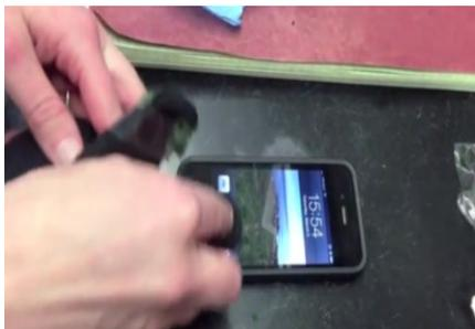
**Step 8:** Test the material by using a set of winter gloves that were not treated with the doped PANI-treated fabric.
