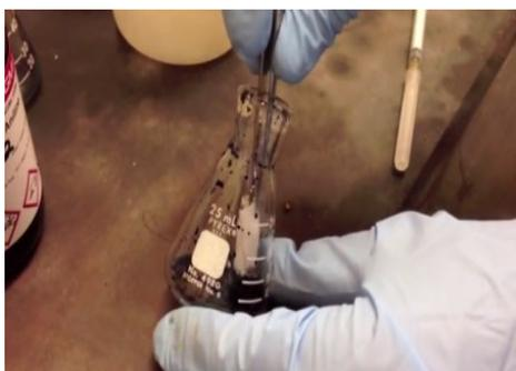
**Step 4:** Using tweezers, dip the small pieces of fabric into the NMP solution with the dissolved polyaniline fibers. The polyaniline solution fully impregnates the fibers of the fabric upon immersion.
