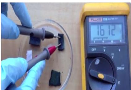
**Step 7c:** Test the freshly doped (wet) PANI-treated fabric. Record result.
