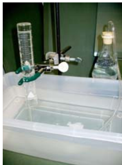
Collecting gas by water displacement
