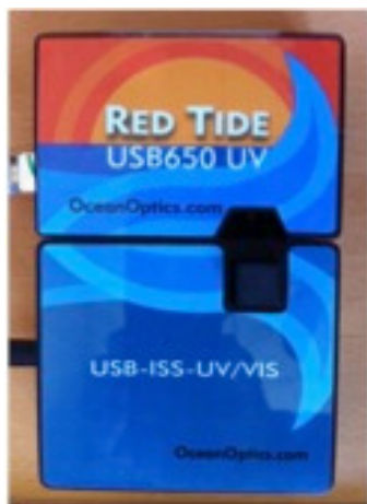
Figure 1: Red Tide USB650 optical bench attached to a USB-ISS-UV-VIS light source and cuvette holder from OceanOptics.
