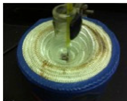
Figure 2: A 25 mL round bottomed reaction flask is clamped into place and inserted into a heating mantle. The CdO and the myristic acid are added to the flask. A 400°C Hg thermometer is inserted into the middle neck. Here we see the reactants before they have melted and reacted.
