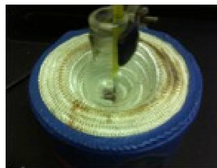
Figure 2: A 25 mL round bottomed reaction flask is clamped into place and inserted into a heating mantle. The CdO and the myristic acid are added to the flask. A 400°C Hg thermometer is inserted into the middle neck. Here we see the reactants before they have melted and reacted.
