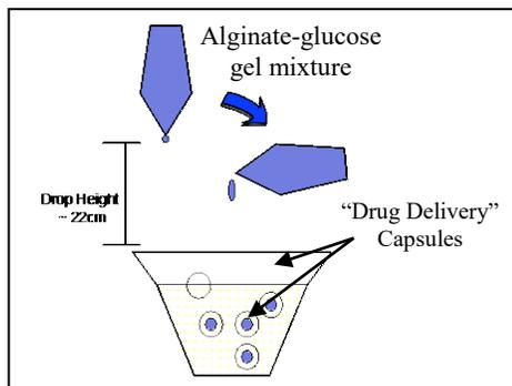
Figure 2. Demonstrating the method for drop formation in CaCl<sub>2</sub>
