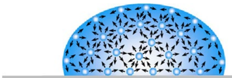
Schematic of surface tension caused by unbalanced forces of liquid molecules at the surface Images from Yuan, Y. and Lee, T.R. (2013) Contact Angle and Wetting Properties. In: Bracco, and Holst, B., Eds., Surface Science Techniques Springer Series, Surface Sciences, Volume 51, Springer Berlin Heidelberg, Berlin and Heidelberg, 3-34. Open Access: https://www.scirp.org/(S(351jmbntvnsjt1aadkpozje))/reference/ReferencesPapers.aspx?Re
